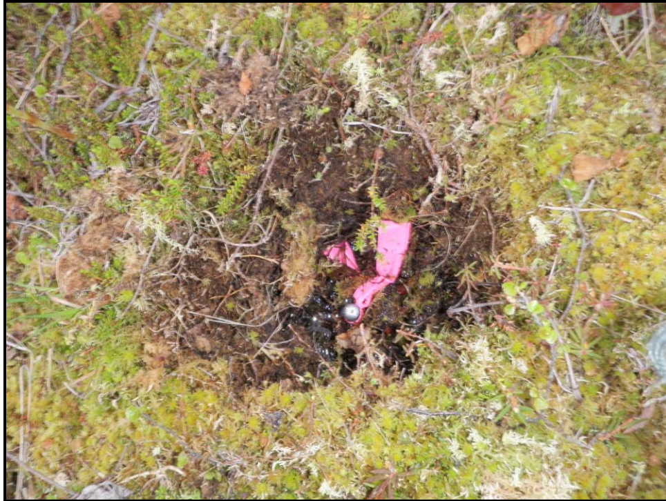
Figure 13 – Monument HK-4. ½ inch x 8 foot steel rod with bullet top.
